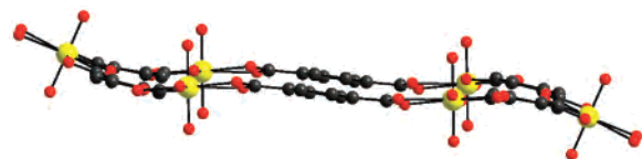
Figure 2. Edge-on view of a single hexagonal unit in 1 showing the chair conformation. U, O, and C atoms are represented by yellow, red, and gray spheres, respectively.
